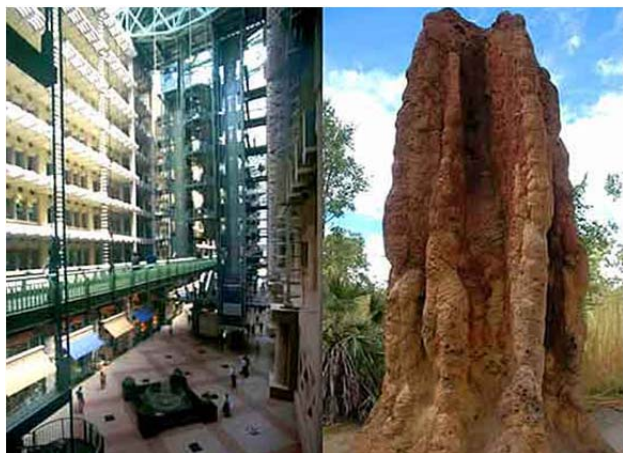
Figure 2.2: Learning's from termite mounds to build temperature controlled buildings in Zimbabwe
